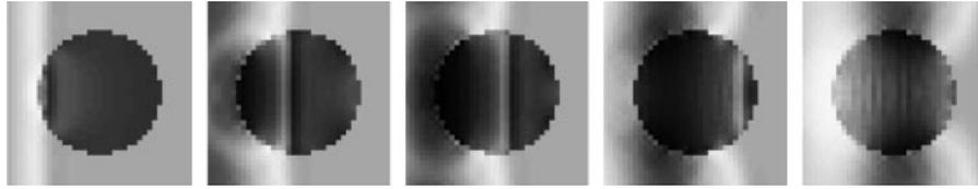
Figure 9. Normalized total pressure around a sphere. Boundary offset  $\alpha = \frac{1}{2}$ . Number of elements along the radius of the sphere  $N_R = 12$ . Plane wave propagates in the direction  $\mathbf{n} = [1, 0, 0]$ . Grid for the sphere indicated with darker shade overlay. Positive pressures are light gray, negative pressures are dark gray.
